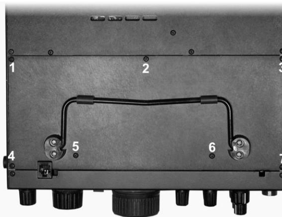
Figure 3. Removing K3 Bottom Cover.
