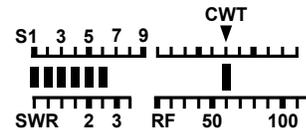
In RTTY modes (**AFSK A** and **FSK D**), mark and space tones are represented by three bars each, with mark to the left of the CWT pointer, and space to the right. When only weak signals are present in the mark/space filters, 1-3 bars will flicker on either side, leading to a “ghosting” effect, as shown here.
