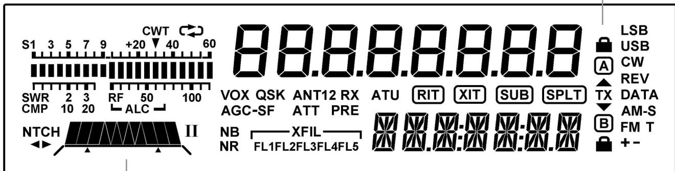
**Filter Graphic:** This shows the approx. bandwidth and position of the receiver's I.F. passband. See **Filter Passband Controls**, pg. 25.
