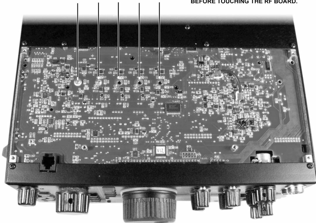
Turn the K3S right side up. Unplug all filters to be repositioned (*those whose mounting screws have been removed*). Lift the filters at each end carefully, first one end then the other, until the connectors separate.
