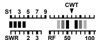
As you tune the VFO close to an RTTY signal, the number of bars will initially increase on one side or the other. Keep tuning until you see a rough balance between left and right bars. (Also see **DTF**, pg. 34, and **CONFIG:TTY LTR**.)
