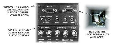
Figure 3. Removing the KIO3 Rear Panel Cover.
