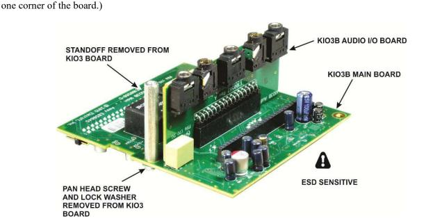
Figure 6. Mounting the Standoff and Audio I/O Board on the KIO3B Main Board.
