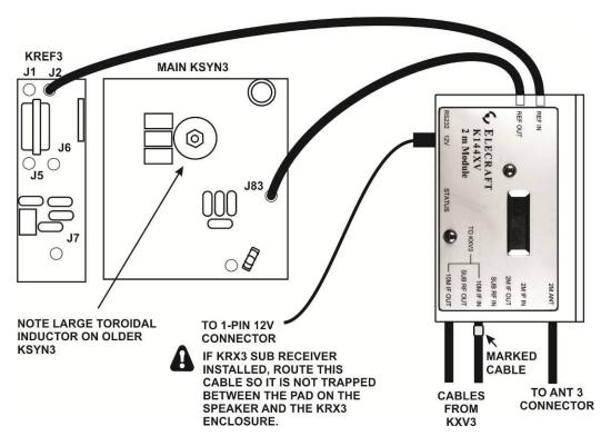
Figure 17. K144XV with K144XV Ref Lock and Original Synthesizers.
