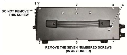
Figure 2. Removing the K3 Left Side Panel.
