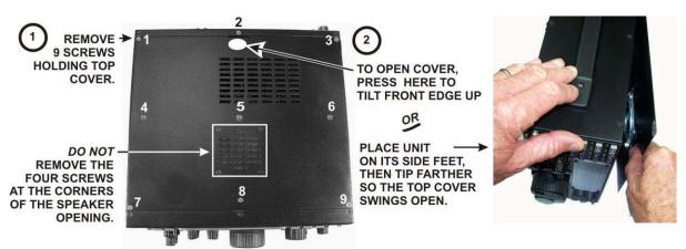
Figure 1. Removing K3 Top Cover.
