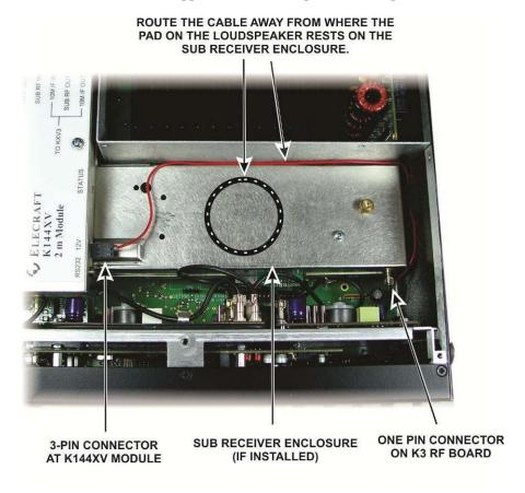
Figure 11. K144XV Power Cable Routing.
