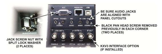
Figure 8. Mounting the new KIO3B Rear Panel Cover.
