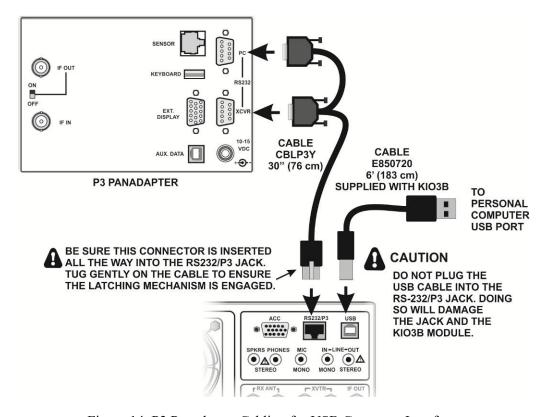
Figure 14. P3 Panadapter Cabling for USB Computer Interface.
