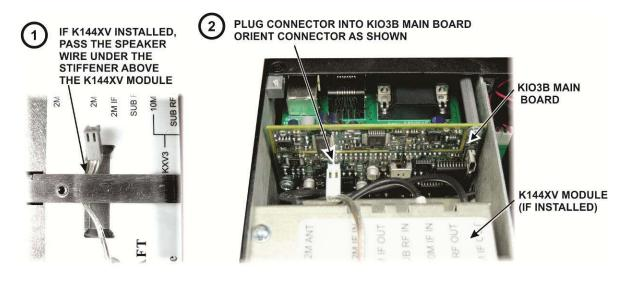
Figure 12. Connecting the Speaker Cable to the KIO3B Board.
