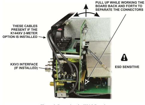
Figure 5. Removing the KIO3 Board.
