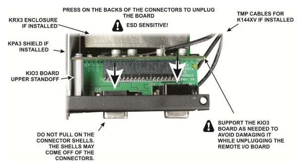
Figure 4. Removing the Remote I/O Board.
