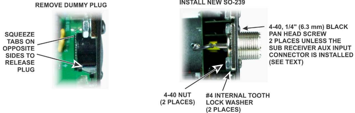
Figure 8. Installing ANT 2 Connector.
