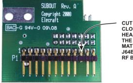
CUT THE THIRD PIN CLOSE TO THE HEADER TO ALLOW THE CONNECTOR TO MATE FULLY WITH J64B ON THE K3 RF BOARD.
