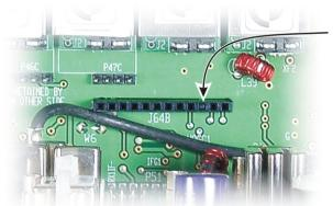
PLACE KEYING INSERT IN THE THIRD HOLE FROM THE END OF J64B AS SHOWN.
