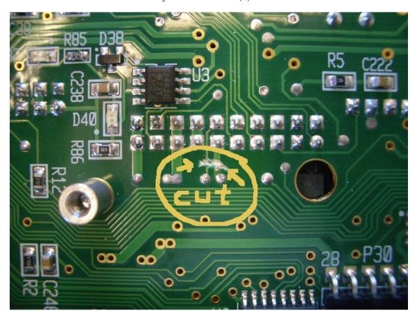
Verify the cuts with an ohmmeter. When you are satisfied the cuts are complete, reinstall the front bottom cover.
