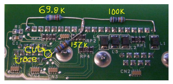
Verify the trace cut by measuring across the 137K resistor. It should measure about 137K ohms.
