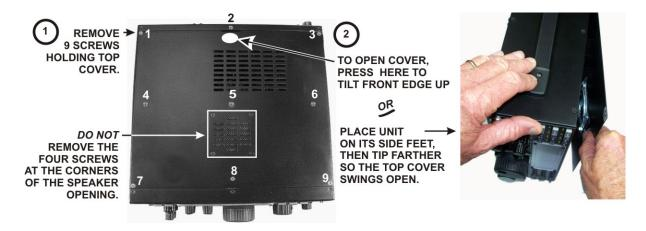
Figure 1. Removing the Top Cover.
