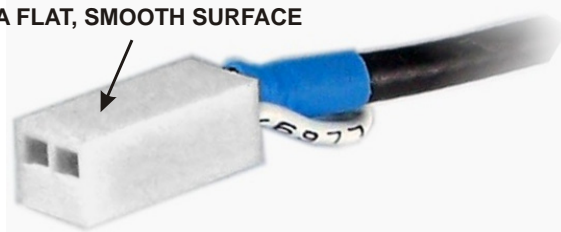
Figure 6. Preparing TMP Cable for Installation.
