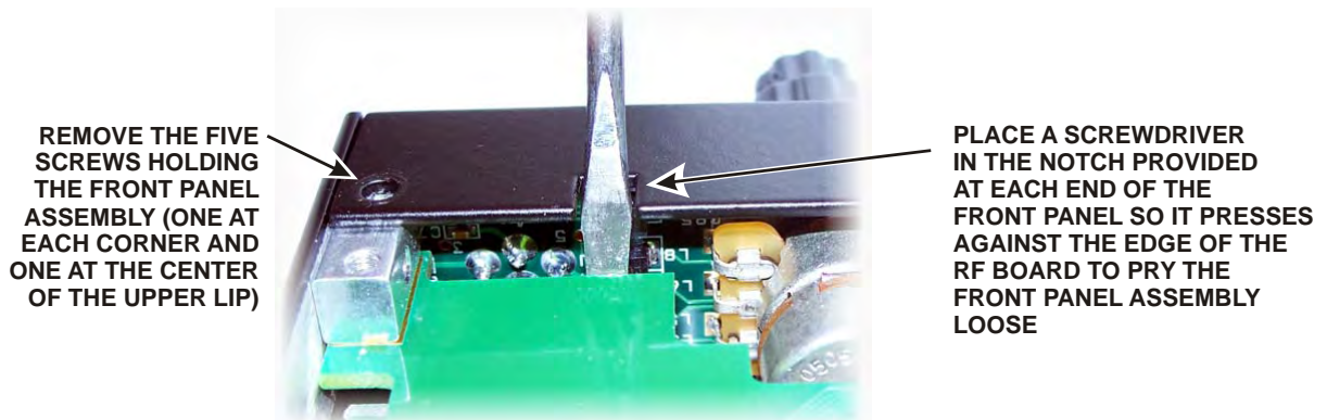
Figure 52. Removing the Front Panel.
