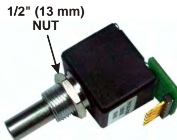
Figure 40. VFO B Encoder Assembly Preparation for Installation.
