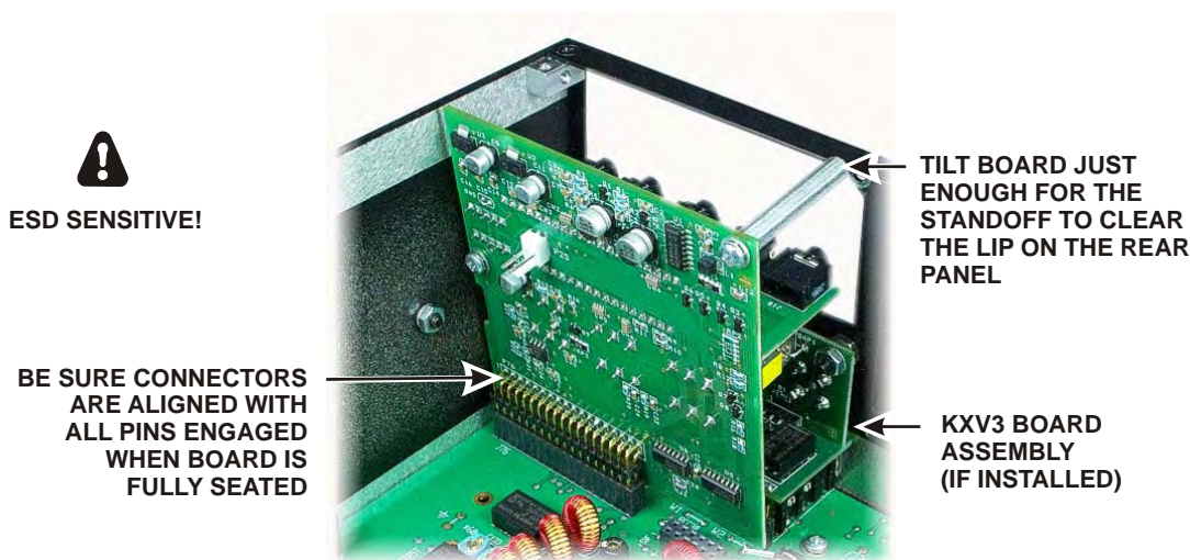
Figure 30. Installing KIO3 Main Board.
