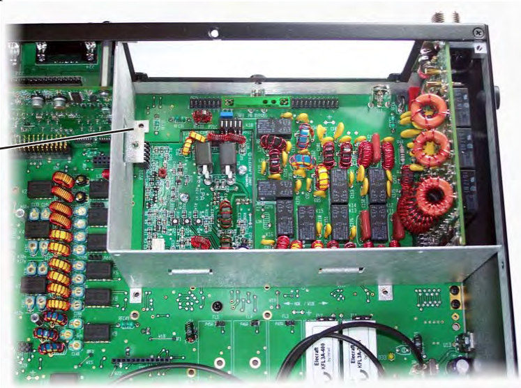
Figure 67. Positioning the KPA3 Shield.
