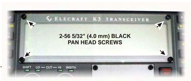
Figure 42. Installing LCD Cover.
