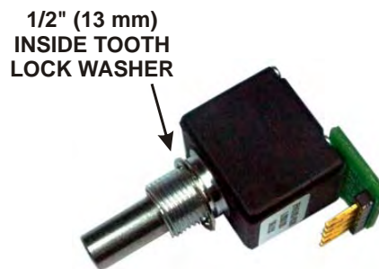
Figure 38. VFO A Encoder Assembly Preparation for Installation.
