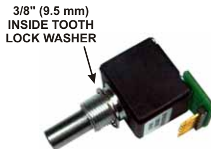
Figure 38. VFO A Encoder Assembly Preparation for Installation.
