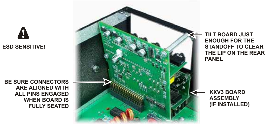
Figure 30. Installing KIO3 Main Board.
