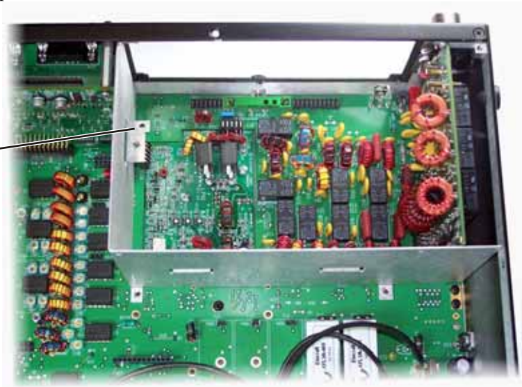
Figure 65. Positioning the KPA3 Shield.
