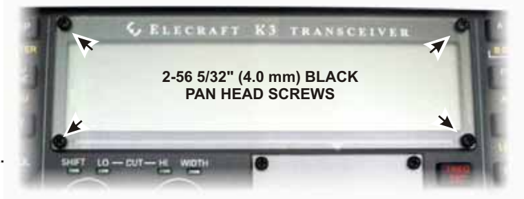
Figure 42. Installing LCD Cover.
