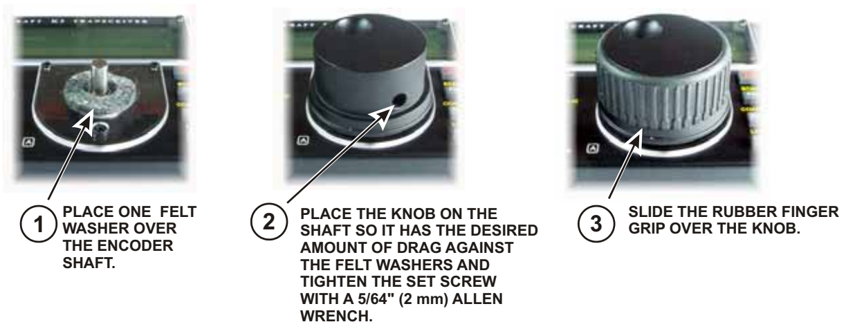
Figure 45. Mounting the VFO A Tuning Knob.
