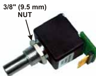
Figure 40. VFO B Encoder Assembly Preparation for Installation.
