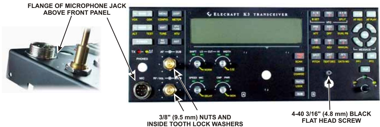
Figure 37. Mounting the Front Panel on the Front Panel Board.
