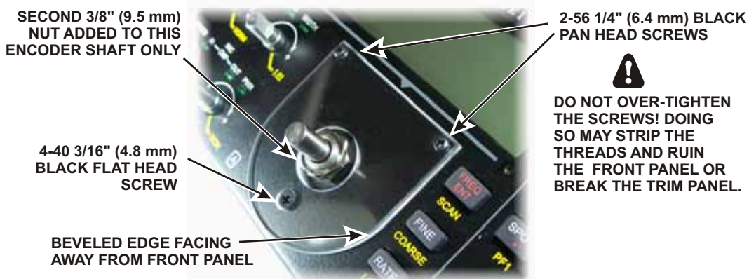
Figure 41. Mounting VFO A Trim Panel.
