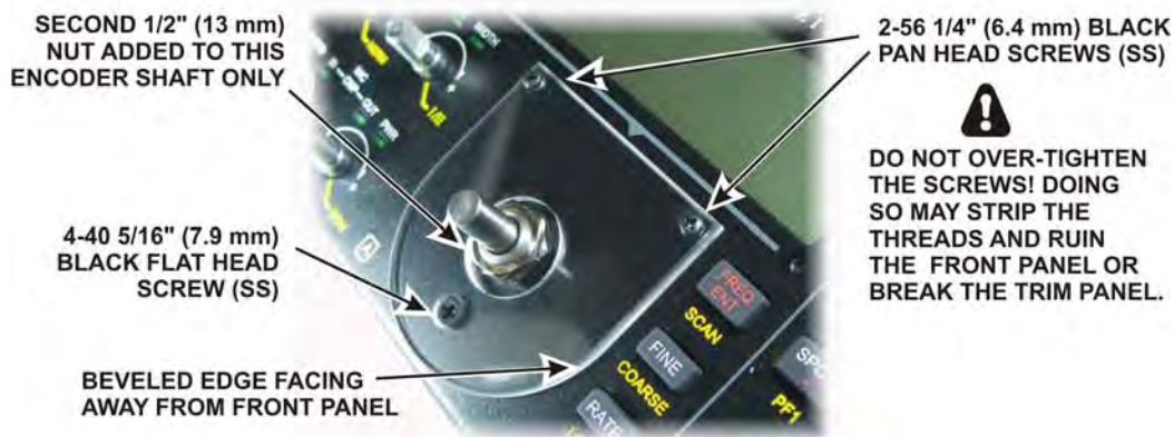
Figure 44. Mounting VFO A Trim Panel.
