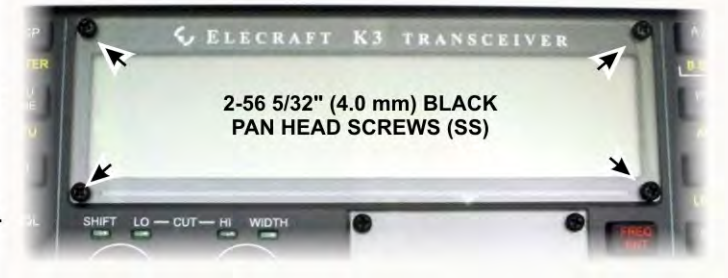
Figure 46. Installing LCD Cover.
