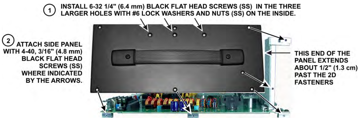
Figure 16. Mounting Left Side Panel.
