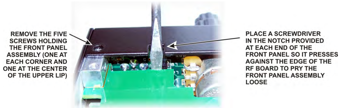
Figure 63. Removing the Front Panel.
