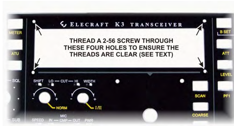
Figure 39. Checking 2-56 Threaded Screw Holes.
