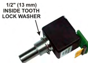
Figure 41. VFO A Encoder Assembly Preparation for Installation.
