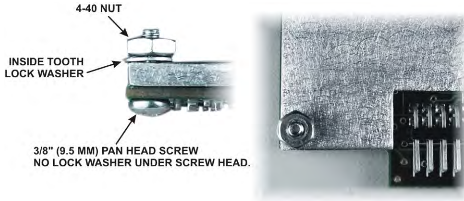
Figure 71 Stiffener Fastener on KSYN3 Board.
