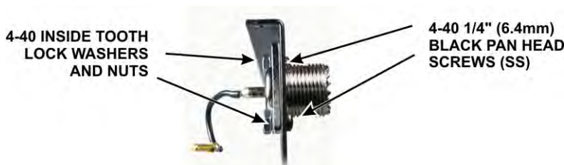
Figure 18. Mounting the ANT1 Connector.
