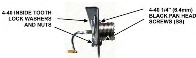
Figure 18. Mounting the ANT1 Connector.
