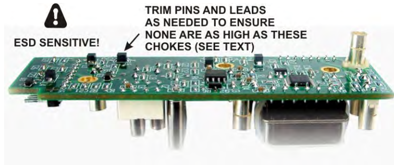
Figure 69. Checking Lead Lengths on KREF3 Board.
