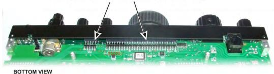
Figure 61. Mounting Front Panel Assembly - Connectors P30 and P35.
