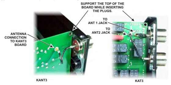
Figure 28. ANT Connections to KANT3 or KAT3 Boards.
