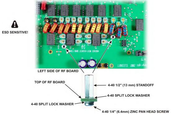
Figure 8. Installing KBPF3 Standoffs.
