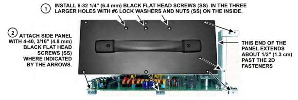
Figure 16. Mounting Left Side Panel.
