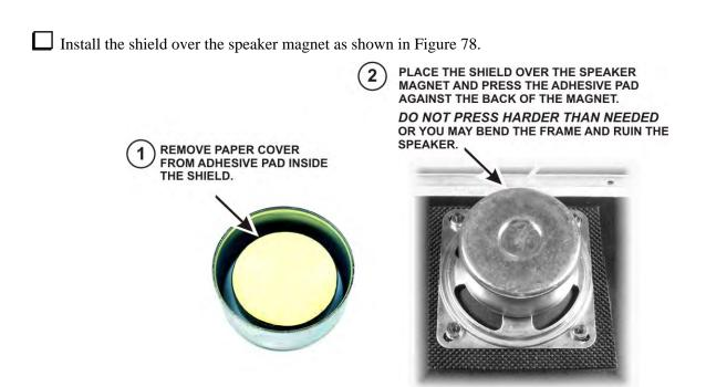
Figure 78. Installing Speaker Magnet Shield.
