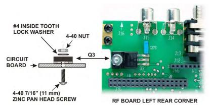
Figure 9. Installing Q3 Hardware.
