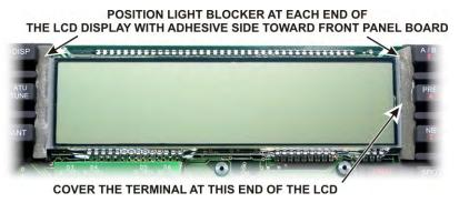
Figure 38. Installing LCD Light Blocker.
