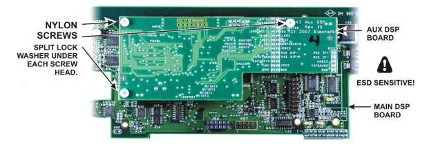
Figure 53. Mating the Main and Auxiliary DSP Boards.
