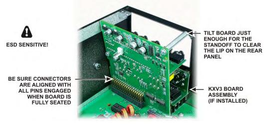
Figure 33. Installing KIO3 Main Board.
