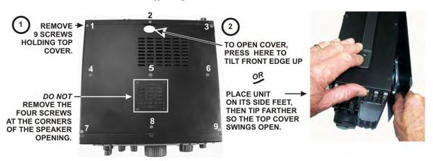
Figure 94. How to Remove the Top Cover.
