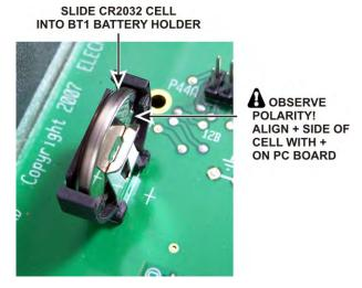
Figure 87. Installing BT1.
