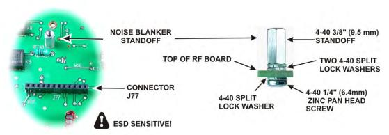
Figure 85. Installing Noise Blanker Standoff.
