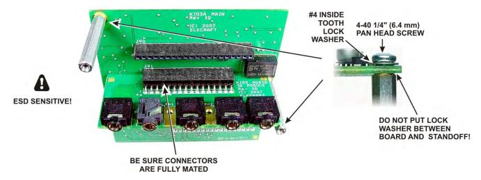
Figure 32. Preparing the KIO3 Board for Installation.
