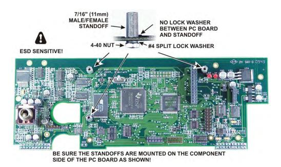
Figure 52. Installing Standoffs on the Main DSP Board.
