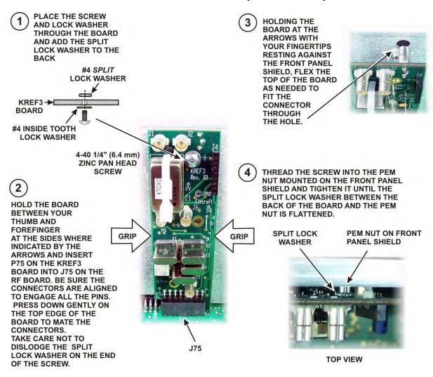
Figure 70. Installing KREF3 Board.
