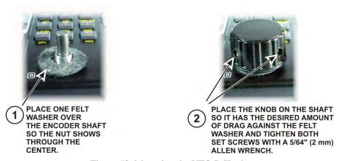
Figure 50. Mounting the VFO B Knob.
