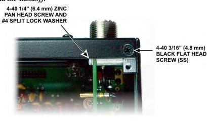
Figure 29. Installing KANT3/KAT3 Mounting Screw.
