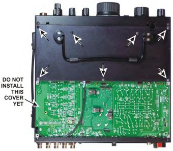
Figure 90. Installing Bottom Cover Forward Section.
