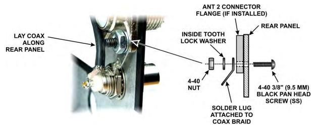
Figure 20. Installing the AUX RF Connector.
