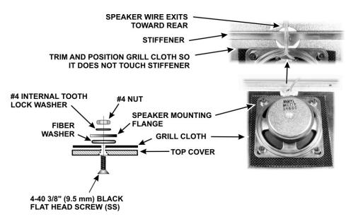
Figure 77. Mounting Loudspeaker.
