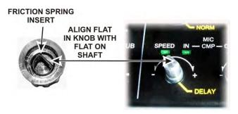
Figure 48. Mounting Friction Knobs.
