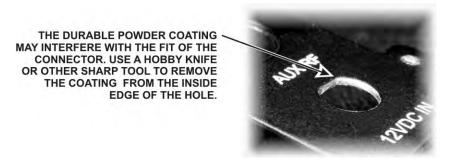
Figure 19. Removing the Powder Coating from the AUX RF Connector Hole.
