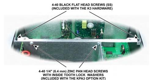
Figure 81. Installing the Chassis Stiffener Bar.
