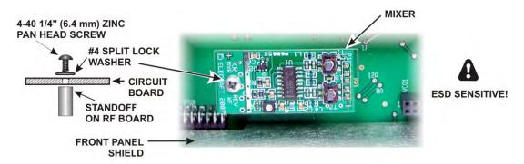
Figure 14. Installing Mixer Board.
