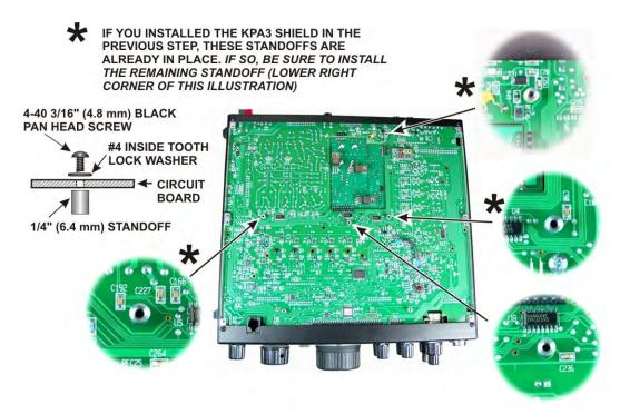
Figure 82. Installing Standoffs on RF Board.
