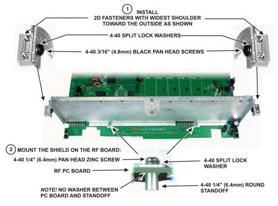
Figure 13. Installing Front Panel Shield.
