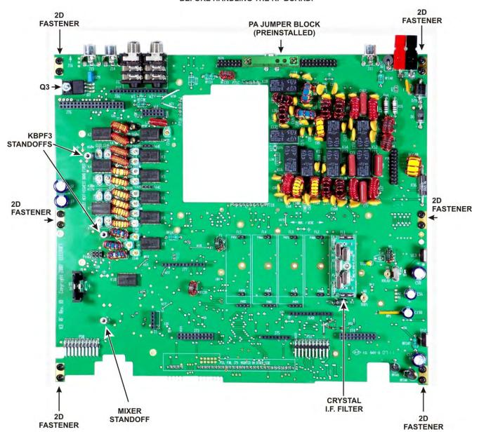
Figure 11. RF Board Partially Assembled.
