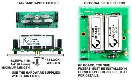
Figure 10. Installing Crystal I.F. Filters.
