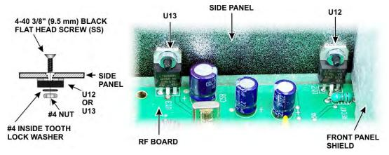
Figure 64. Attaching U12 and U13 to the Right Side Panel.
