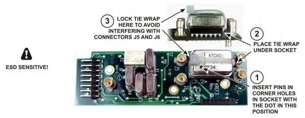
Figure 68. Mounting TCXO Module on KREF3 Board.
