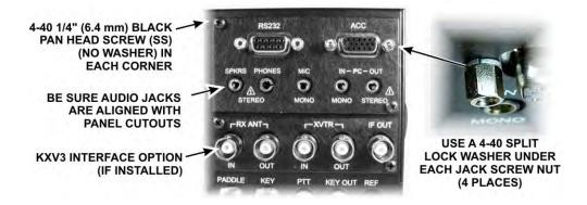
Figure 35. Mounting the KIO3 Connector Panel.
