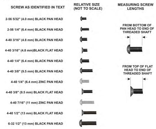
Figure 2. Screw Sizes Used in Assembly.
