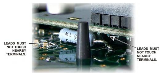
Figure 57. Checking the Position of R3.
