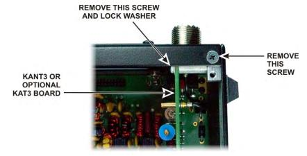
Figure 60. Removing Right Side Panel Hardware.
