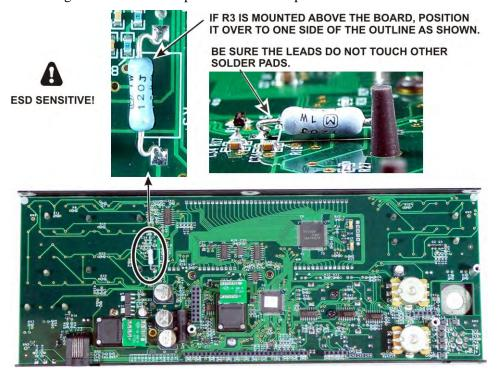
Figure 54. Positioning R3 on the Front Panel Board.
