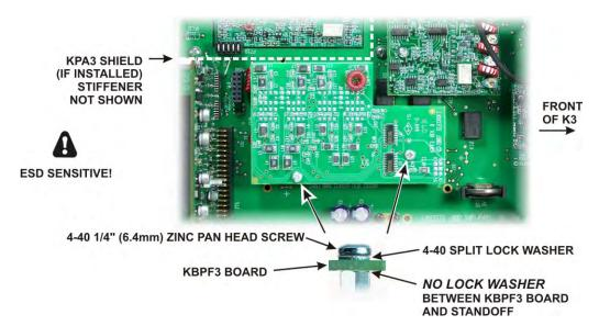
Figure 88. Installing the KBPF3 Option Board.
