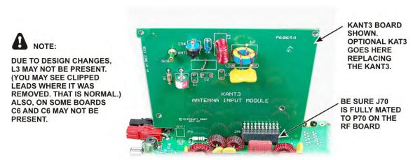
Figure 24. Installing the KANT3 or KAT3 Board.
