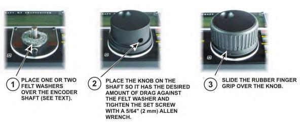
Figure 49. Mounting the VFO A Tuning Knob.
