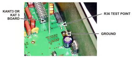
Figure 65. R36 Test Point.
