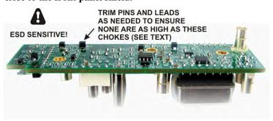
Figure 69. Checking Lead Lengths on KREF3 Board.
