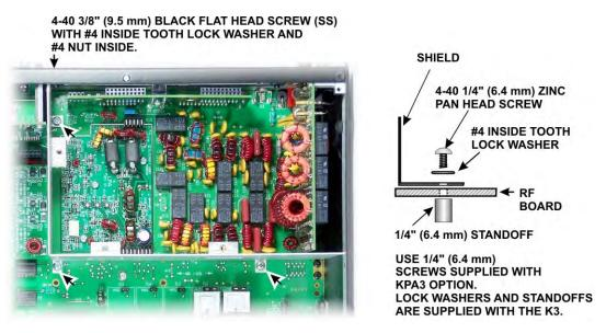
Figure 80. Attaching the KPA3 Shield.
