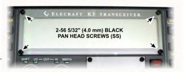
Figure 46. Installing LCD Cover.
