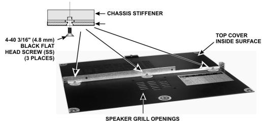
Figure 76. Attaching Chassis Stiffener to Top Cover.
