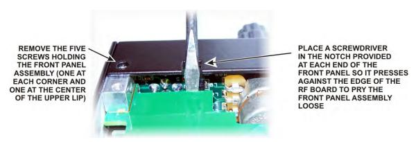
Figure 63. Removing the Front Panel.
