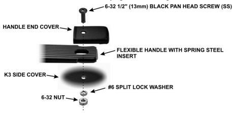
Figure 15. Installing Side Handle Mounting Hardware.
