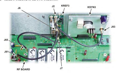
Figure 75. Installing KREF3 TMP Cables.
