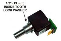
Figure 41. VFO A Encoder Assembly Preparation for Installation.
