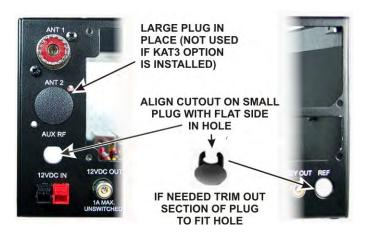
Figure 30. Installing Rear Panel Hole Plugs.
