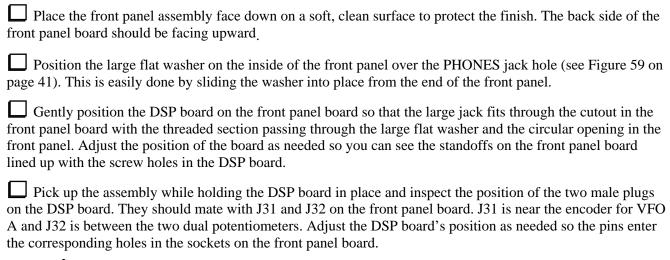
**A** Use a strong light to look between the boards to be sure the connectors are properly mated. Be especially careful to check the connector near the dual potentiometers. Be sure the pins are entering the socket and not resting alongside it.
