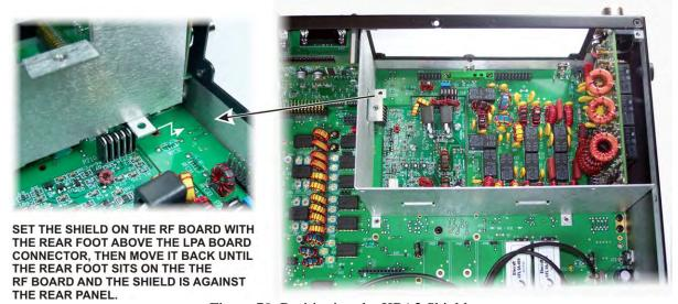
Figure 79. Positioning the KPA3 Shield.
