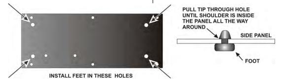
Figure 21. Installing Side Panel Feet.
