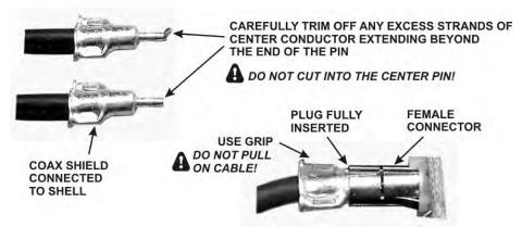
Figure 74. TMP Cable Connectors.
