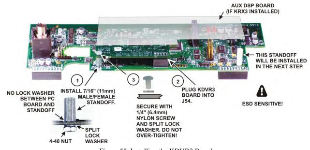
Figure 55. Installing the KDVR3 Board.
