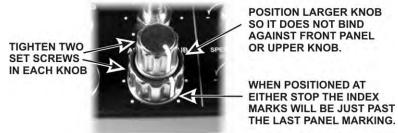
Figure 47. Mounting Concentric Knobs.
