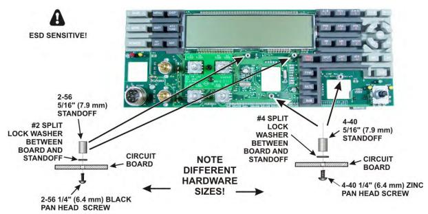
Figure 37. Preparing the Front Panel Board for Mounting, Part 2.
