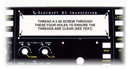
Figure 39. Checking 2-56 Threaded Screw Holes.
