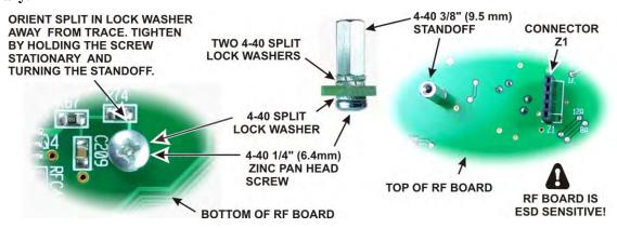
Figure 7. Installing Mixer Standoff.
