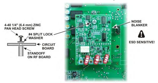
Figure 86. Installing the Noise Blanker Board.
