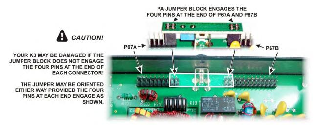
Figure 89. Installing the PA Jumper Block.
