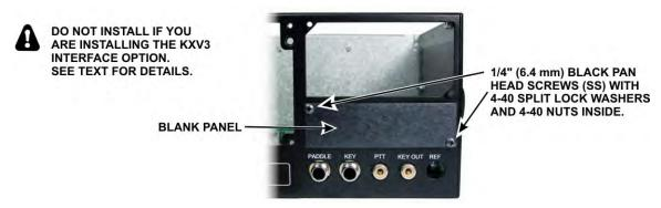
Figure 31. Preparing Rear Panel for KIO3 Installation.
