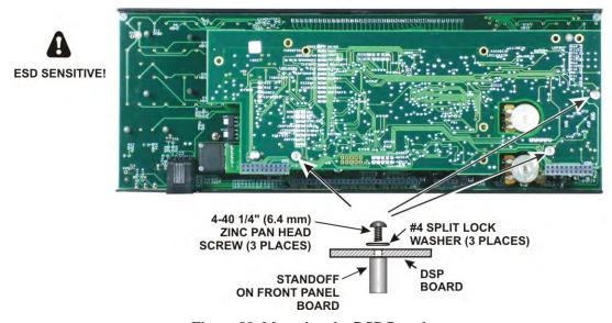
Figure 58. Mounting the DSP Board.
