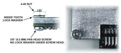
Figure 71 Stiffener Fastener on KSYN3 Board.
