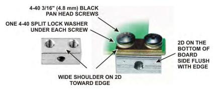
Figure 6. Installing 2D Fasteners on RF Board.
