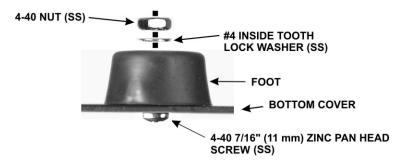
Figure 84. Installing Rear Feet.
