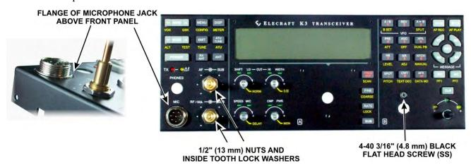
Figure 40. Mounting the Front Panel on the Front Panel Board.
