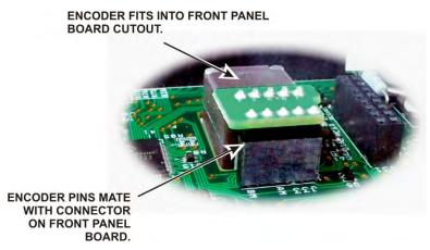
Figure 42. Mounting VFO Encoders.
