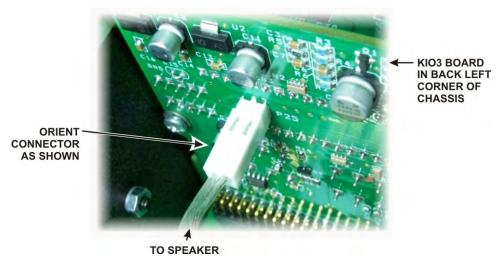
Figure 93. Connecting Speaker to KIO3 Board.
