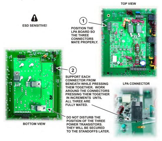
Figure 12. Installing the Low Power Amplifier (LPA).
