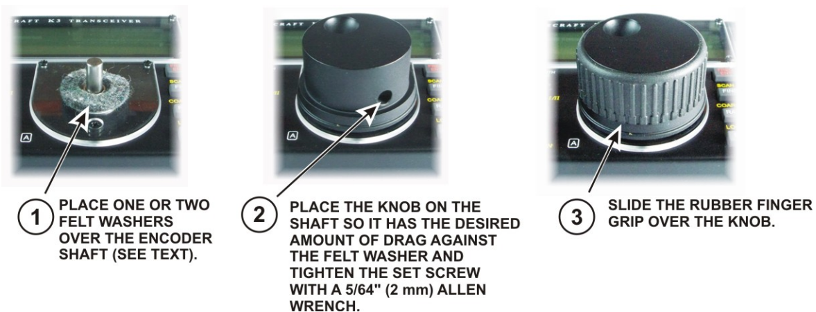
Figure 49. Mounting the VFO A Tuning Knob.
