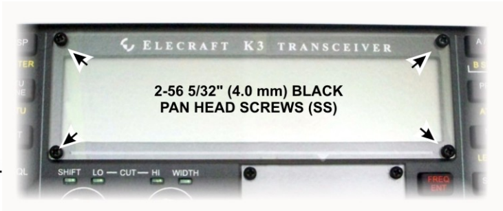
Figure 46. Installing LCD Cover.
