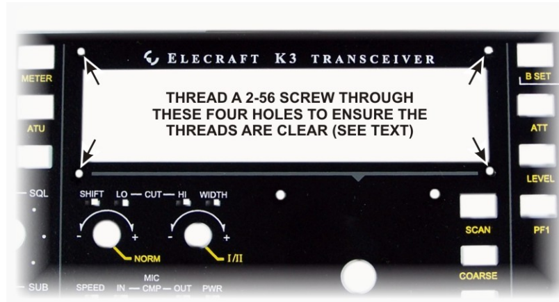
Figure 39. Checking 2-56 Threaded Screw Holes.
