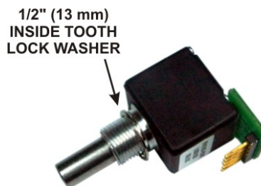
Figure 41. VFO A Encoder Assembly Preparation for Installation.
