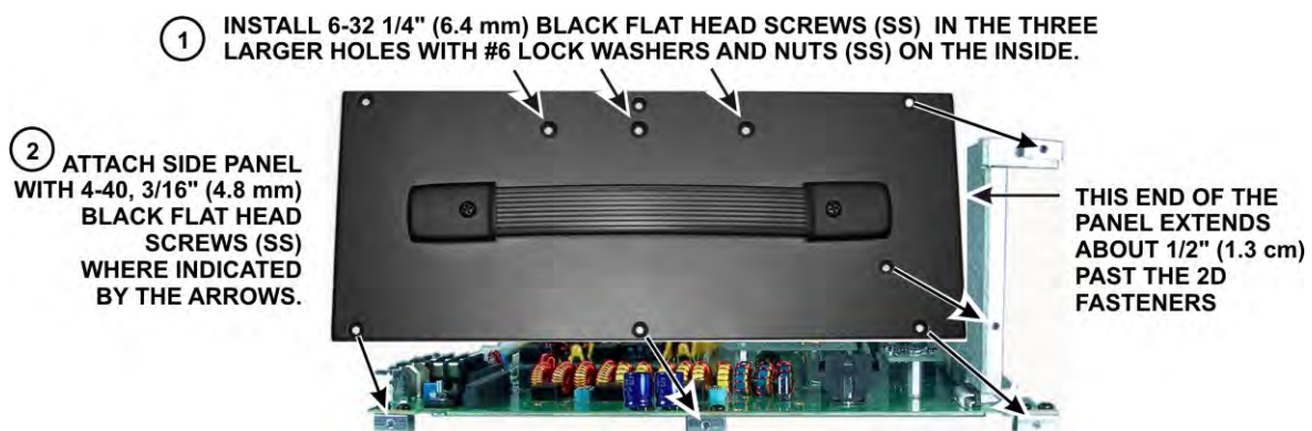
Figure 16. Mounting Left Side Panel.
