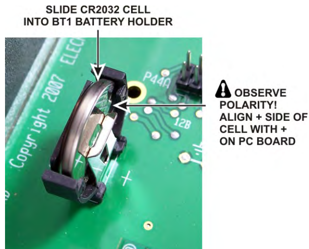
Figure 87. Installing BT1.
