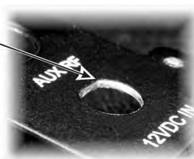
Figure 19. Removing the Powder Coating from the AUX RF Connector Hole.
