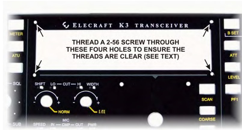
Figure 39. Checking 2-56 Threaded Screw Holes.
