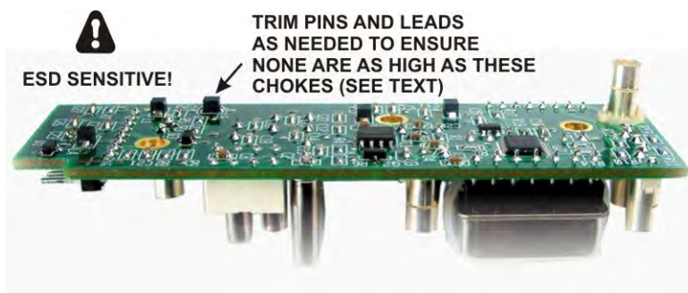
Figure 69. Checking Lead Lengths on KREF3 Board.
