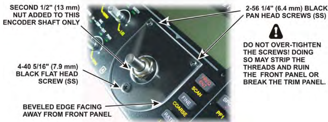
Figure 44. Mounting VFO A Trim Panel.
