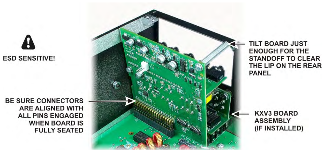
Figure 33. Installing KIO3 Main Board.
