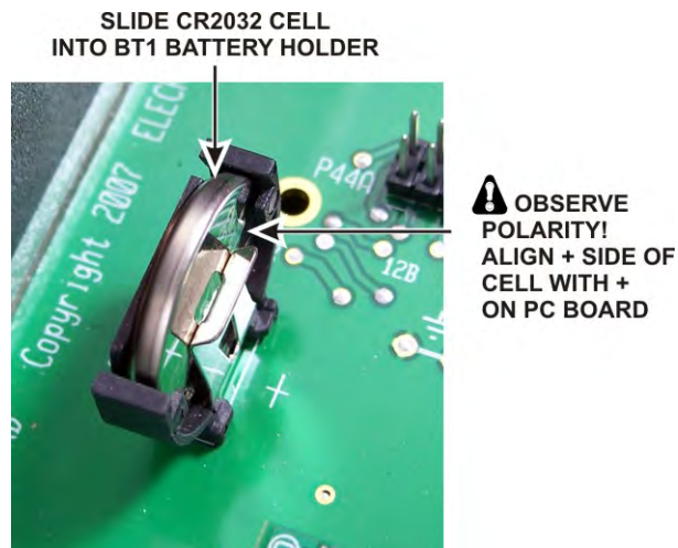
Figure 87. Installing BT1.
