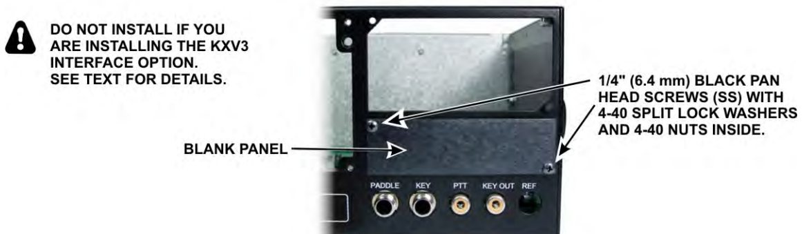
Figure 31. Preparing Rear Panel for KIO3 Installation.
