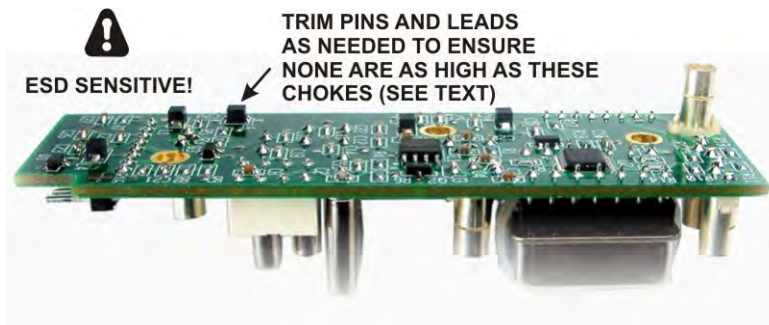
Figure 69. Checking Lead Lengths on KREF3 Board.
