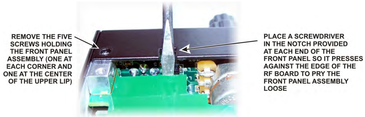
Figure 63. Removing the Front Panel.
