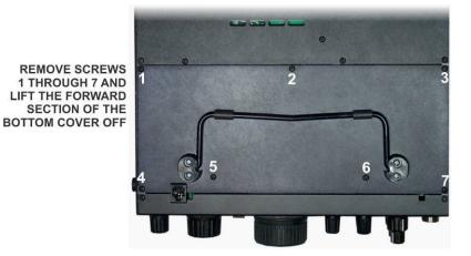
Figure 11. Removing Bottom Cover Front Section.
