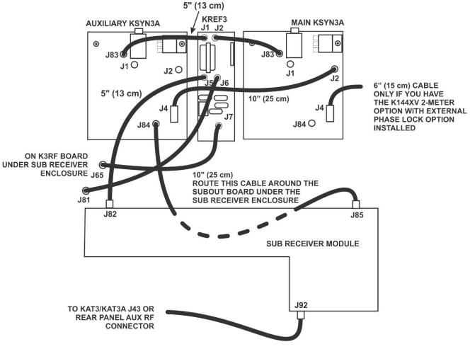
Figure 19. TMP Cable Routing.
