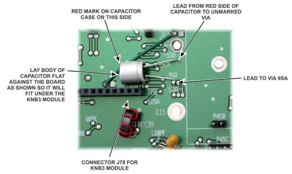
Figure 9. Mounting the Poly Capacitor on the Sub Receiver Main Board.
