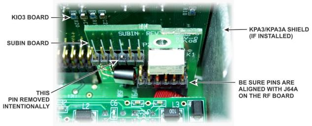
Figure 17. Replacing the SUBIN Board.
