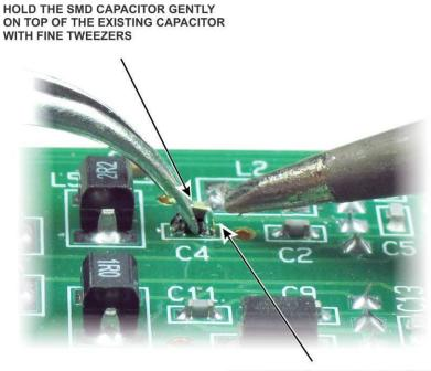
BRIEFLY TOUCH THE END OF BOTH CAPACITORS WITH A TINNED HOT SOLDERING IRON TO JOIN THEM TOGETHER
