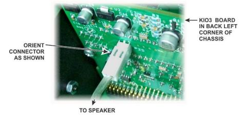
Figure 22. Connecting Speaker Cable.
