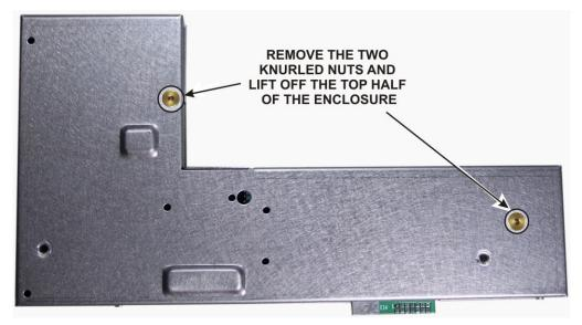
Figure 7. Removing the Top of the Sub Receiver Enclosure.
