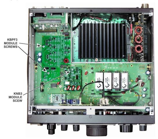
Figure 10. KBPF3 and KNB3 Modules on K3 RF Board
