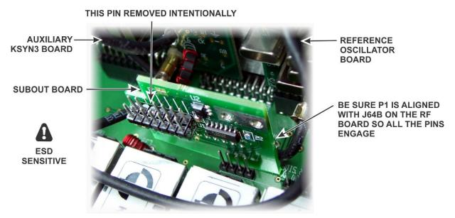
Figure 18. Replacing the SUBOUT Board.
