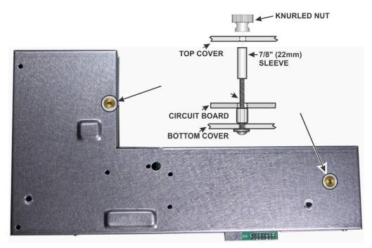
Figure 15. Replacing the Sub Receiver Top Cover.
