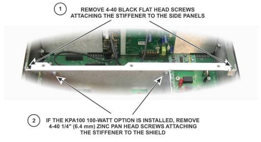
Figure 2. Chassis Stiffener Bar.
