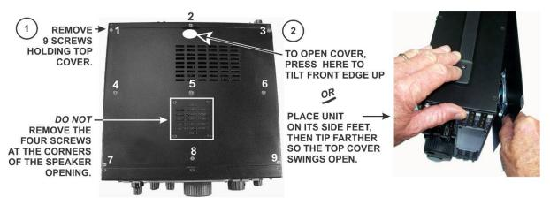
Figure 1. Removing K3 Top Cover.
