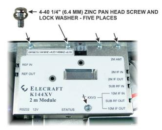
Figure 3. Removing the K144XV 2 Meter Module.
