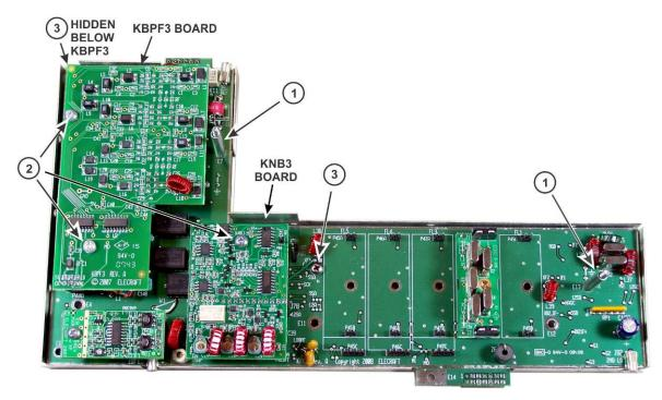
Figure 8. Removing the Main Board from the Enclosure.
