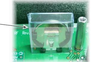
Figure 6. Removing the Battery Cover.
