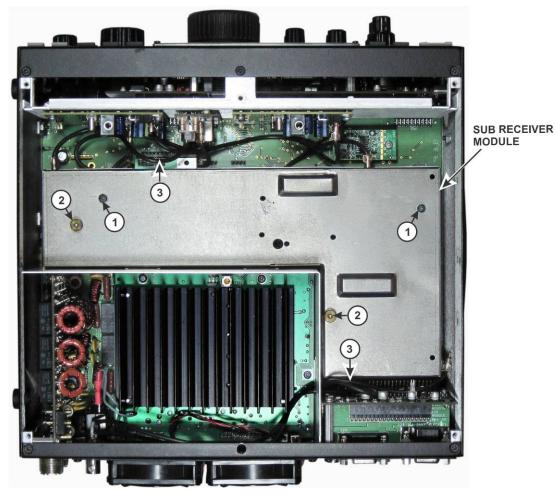
Figure 5. Removing the KRX3 or KRX3A Module.
