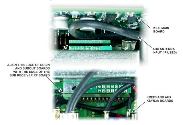
Figure 20. Aligning the Sub Receiver Module Connectors with the SUBIN and SUBOUT Interface Boards.
