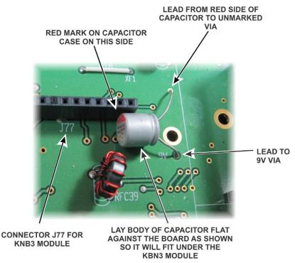
Figure 12. Mounting the Poly Capacitor on the K3 RF Board.
