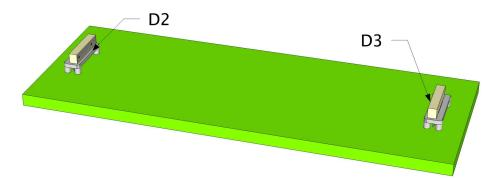
While holding the LED (D2) and its spacer firmly in place, use your soldering iron to apply a small amount of solder to one of the two pins.
