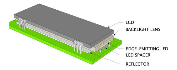
Locate the bag labeled **K2 Backlight**. Included in the bag should be the following:
