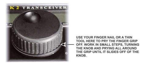
Figure 5. Removing the Finger Grip.
