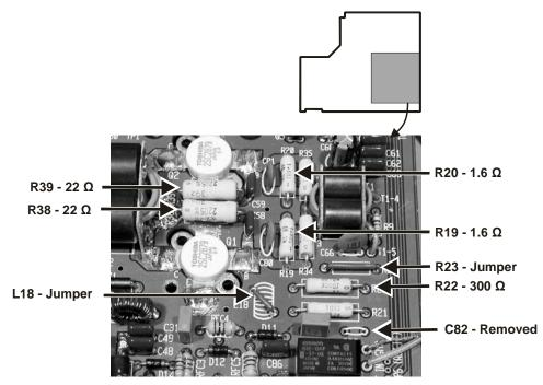
Figure 2. Input and Feedback Circuit Component Changes.
