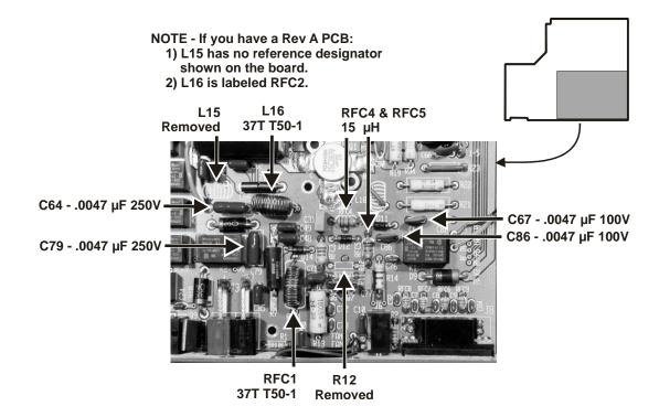
Figure 5. T/R Switch Components.
