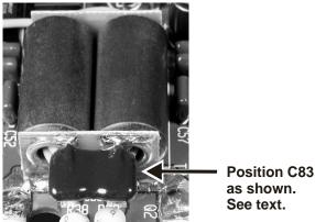
Figure 4. Installing C83.
