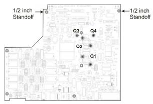
Figure 1. Removing the KPA100 PCB.
