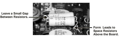
Figure 3. Installing R38 and R39.
