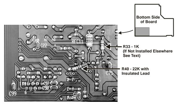
Figure 8. Installing R33 and R40.
