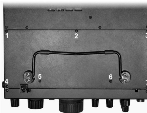
Figure 3. Removing K3 Bottom Cover.
