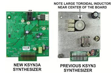
**Page 8:** If your K3 has the new KSYN3A synthesizer, only one TMP coaxial cable is used as shown below. Do not connect a cable to the KREF3 board as shown in Figure 4 in the manual.
