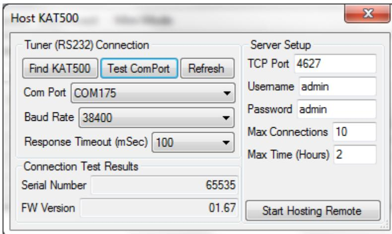
This dialog allows you to configure the com port, baud rate required to communicate with your KAT500. It also allows you to setup the Server details for hosting your KAT500 over the network.
