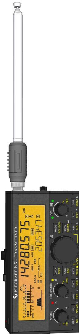
The Elecraft AX2 is a miniature 20 meter telescoping whip that disassembles into a 6" (15 cm) whip and 2.5" (6 cm) base unit. **It is intended to be used with an ATU (antenna tuner).**
