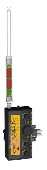
The Elecraft AX1 is a compact telescoping whip that disassembles into 6" (15 cm) pieces, so it will fit into small "grab & go" bags... or your back pocket. On the basic unit, a two-position switch selects 20 meters (resonant) or 17/15 meters (a low-loss match can be achieved using an antenna tuner on both bands). The AXE1 Extender (pg. 7) adds 40 and 30 meter coverage (ATU required).
