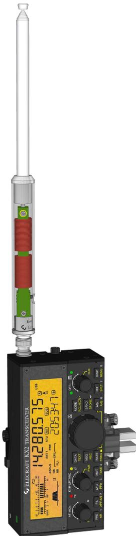
The Elecraft AX1 is a compact telescoping whip that disassembles into 6" (15 cm) pieces, so it will fit into small “grab & go” bags... or your back pocket. On the basic unit, a two-position switch selects 20 meters (resonant) or 17/15 meters (a low-loss match can be achieved using an antenna tuner on both bands). The AXE1 Extender (pg. 7) adds 40 and 30 meter coverage (**ATU required**).
