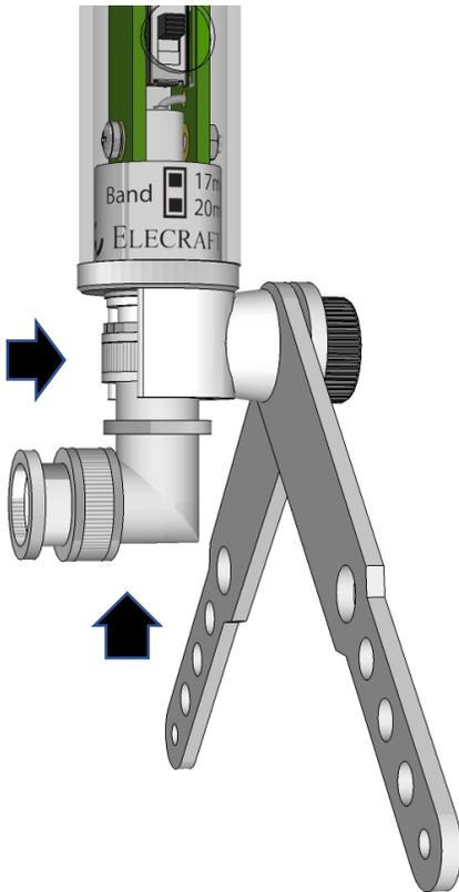
**NOTE:** The legs of the AXB1 may not be in electrical contact with the whip's BNC connector, so they should not be used as a radial wire attachment point.
