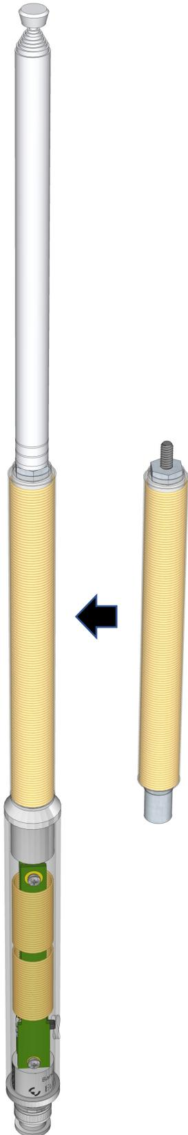
The AXE1 extender allows the AX1 to be used on 40 and 30 meters. It adds 6 inches (15 cm) of overall length. **AN ANTENNA TUNER IS REQUIRED ON 40 AND 30 METERS BECAUSE THE AX1 WHIP + AXE1 EXTENDER IS VERY NARROW BANDED.** See setup and matching instructions below.
